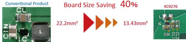
High-growth focus product: Inductor Built-in Micro DC/DC converters
